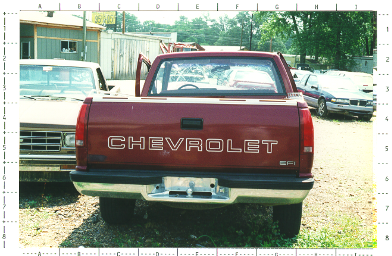
# 74 -- Back view of 1988 Chevrolet C-1500 pickup showing undamaged back side; NOTE: driver's door window frame is bent outwards
